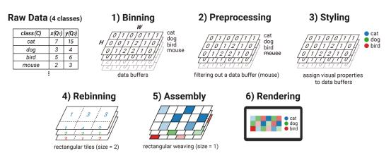
Fig. 3: The six stages of the Class Buffer model.
